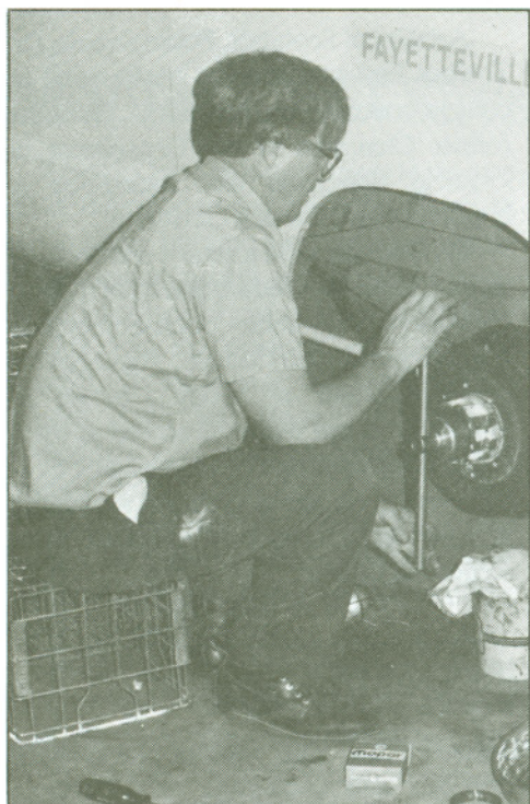
Billy Bain replaces a wheel bearing on a college van.
